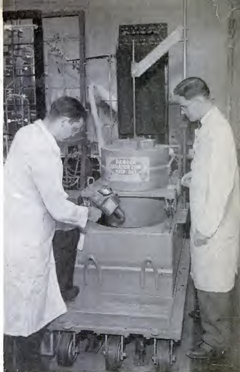
Seven tons of lead shield a piece of irradiated cobalt no bigger than your index finger in this rolling material-testing machine, checked with a radiation counter for possible gamma-ray danger
